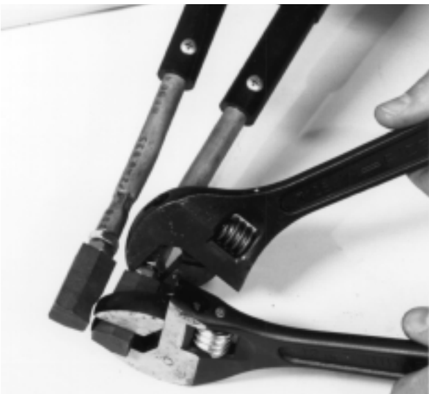
Figure 8 – Removing Carbon Tips
